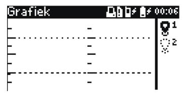
The selected zone (🕏) for which the graph is shown can be seen on the right. Pressing the required zone will show its values on the graph.
