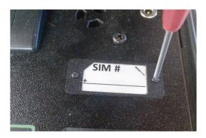
Push the holder to the left so that it can be moved upwards:
