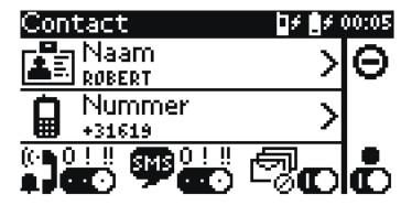
Enter the name and telephone number by pressing the relevant field. In order to check the functionality, a test text message will be sent to the number when a telephone number is added.
