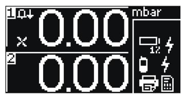
The right-hand side of the screen shows the status. When an alarm situation occurs, the circon appears and the AMS PM will give an audible alarm signal. Pressing the icon accepts the alarm and the alarm signal is suppressed.
