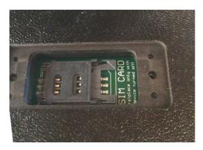
Place the SIM card in the holder and let it drop down again. Sliding the holder to the right fixes the SIM card:
